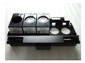
Slide the holder on the filter module to the right to close the filter module.
