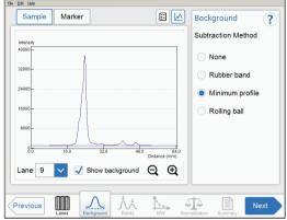
Rolling Use this option to subtract the background below the graph as if erasing it using the radius of a ball. A small radius will subtract more background than a large.
