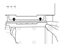
2 Push the attachment upward firmly into the guide until you hear a clicking sound.
