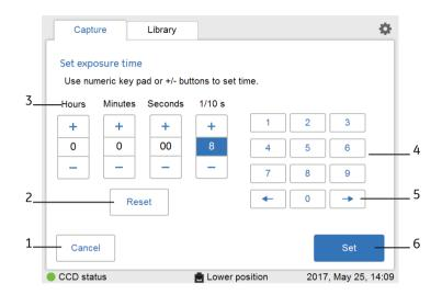
**Note:** The time displayed in the **Set exposure time** window, is by default the exposure time used during the last capture. The time can be set from 0.1 seconds up to 10 hours.
