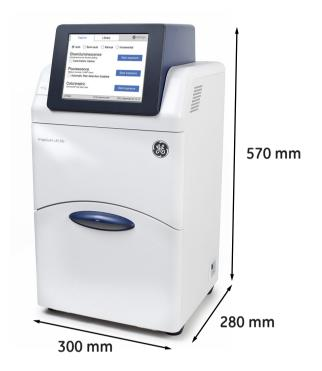
The ImageQuant LAS 500 imager weighs 15 kg.
