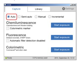
2 Check the **Automatic filter detection disabled box**, if the fluorescence sample is larger than the image area (10×15 cm) or if the automatic filter detection fails.
