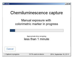
When the exposure is finished the image view appears displaying the image. ImageQuant LAS 500 creates a folder containing image files that can be saved. For details see *File formats, on page 109*.
