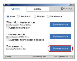
*Result*: The exposure will begin following a pre-exposure. A progress bar appears on the screen indicating the time remaining of the imaging process, the exposure selected and the actual exposure time.
