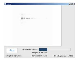
Result: The number of images matching the selected repetitions are displayed as they are exposed. A progress bar indicates the time remaining for imaging.
