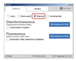
2 Check the **Automatic filter detection disabled** box, if the fluorescence sample is larger than the image area (10×15 cm) or if the automatic filter detection fails.
