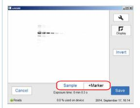
Incremental exposure displays a series of images one at a time as they are exposed. Navigate among the images using forward and backward arrows.
