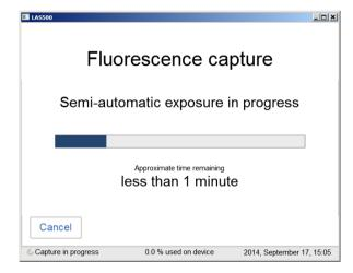
When the exposure is complete, image view appears and the image are displayed. ImageQuant LAS 500 creates a folder containing the image files that can be saved. For details see *File formats, on page 109*.
