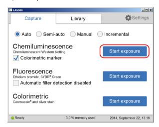
*Result*: Exposure starts after pre-exposure and a progress bar appears on the screen. This indicates the remaining time for the imaging process, the exposure selected and the actual exposure time.
