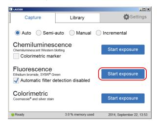
Result: The exposure will begin following a pre-exposure. A progress bar appears on the screen indicating the time remaining of the imaging process, the exposure selected and the actual exposure time.
