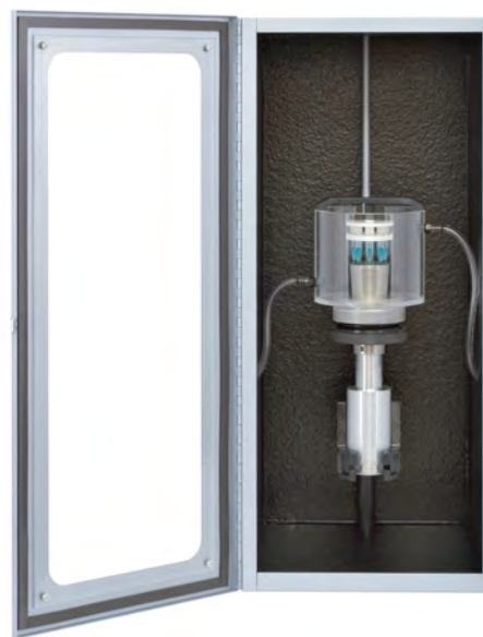
432B2 shown with cup horn (Cup horn sold separately.)
