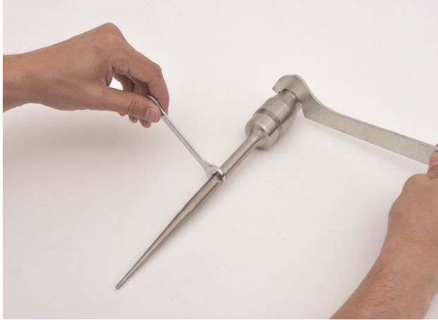
Replacement Tip Removal
