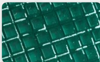
Figure 3: Competitor's plate showing areas with no adhesive
