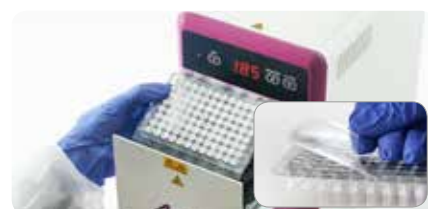
Figure 2: Random Access Sealing Procedure using the 4s3™ Semi-Automated Sheet Heat Sealer (4ti-0655)
