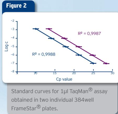
Both plates showed comparable assay efficiencies of 81 and 82% as can be seen from the equal slope of both graphs.
