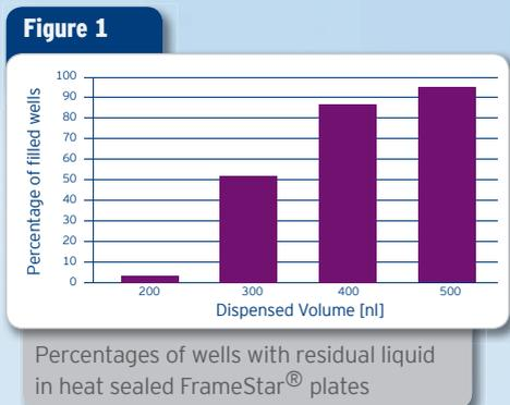
At 500nl over 95% of the wells show tartrazine still in solution, at 400nl almost 90% of the wells remain filled. At 300nl half of the wells are empty. 200nl volumes are almost completely evaporated. Thus, we conclude the average loss of water during a standard PCR to be between 100 and 300nl.
