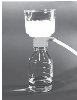
Figure 1: Correct use of the NucleoBond® Bottle Top Filter
